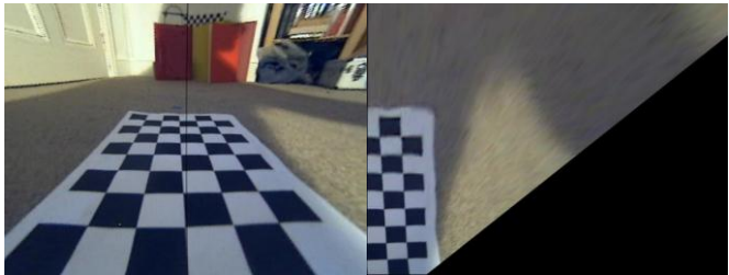
Figure 3: visual representation of Pre and Post perspective transformation
