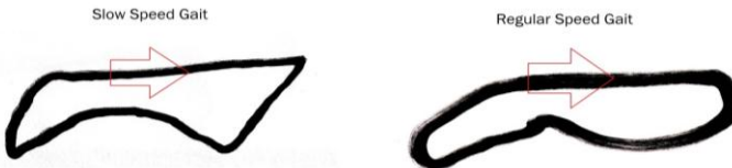
Figure 6: Foot trajectory drawn by the New gait. On the left the robot is set to 80 poses per cycle and 3 ticks per pose, while on the right to 24 poses per cycle and 3 ticks per pose. Stride length is 20 and stride height is 10.
