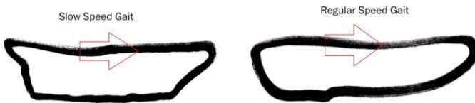
Figure 5: Foot trajectory drawn by the Half-Triangular gait. On the left the robot is set to 80 poses per cycle and 3 ticks per pose, while on the right to 24 poses per cycle and 3 ticks per pose. Stride length is 20 and stride height is 10.
