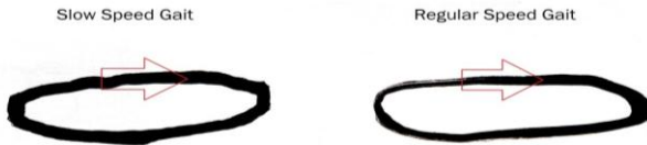
Figure 1: Foot trajectory drawn by the circular gait. On the left the robot is set to 80 poses per cycle and 3 ticks per pose, while on the right to 24 poses per cycle and 3 ticks per pose. Stride length is 20 and stride height is 10.
