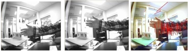
Figure 2: A simple example of optic flow, the third image represents the optic flow vectors (red lines)
