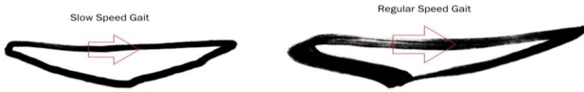
Figure 2: Foot trajectory drawn by the Triangular gait. On the left the robot is set to 80 poses per cycle and 3 ticks per pose, while on the right to 24 poses per cycle and 3 ticks per pose. Stride length is 20 and stride height is 10.
