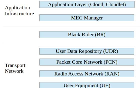
Fig. 4. Reference-Architecture of the MEC Manager
