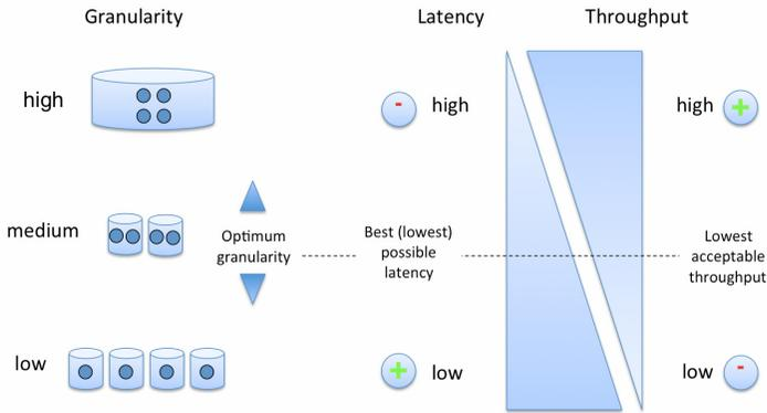
**Figure 6: Throughput and latency depend on data granularity**
