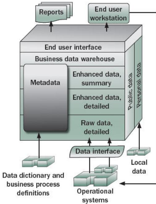
**Figure 2: Data warehouse architecture (Devlin, 1988)**
