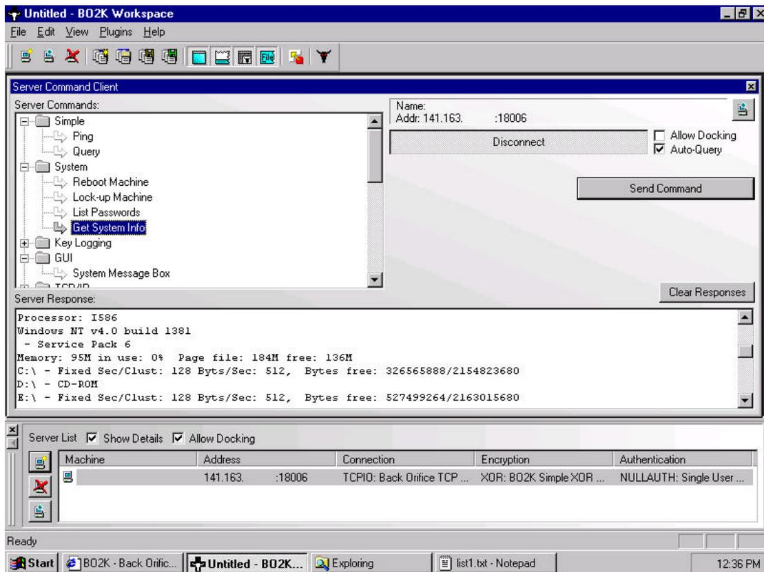
**Figure 1 : The Back Orifice 2000 administration tool**
