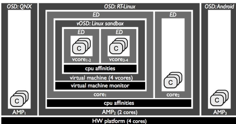
**Figure 4: Exemplary composition of different containment techniques.**
