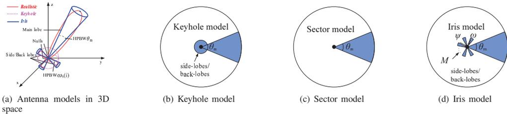
Fig. 1. Directional Antenna Models
